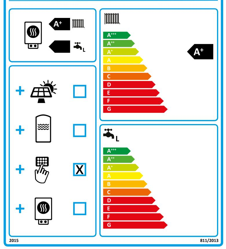
Product datasheet: Composite system consisting of room heater and temperature controller to regulation (EU) no. 811/2013 / (S.I. 2019 No. 539 / Schedule 2)
