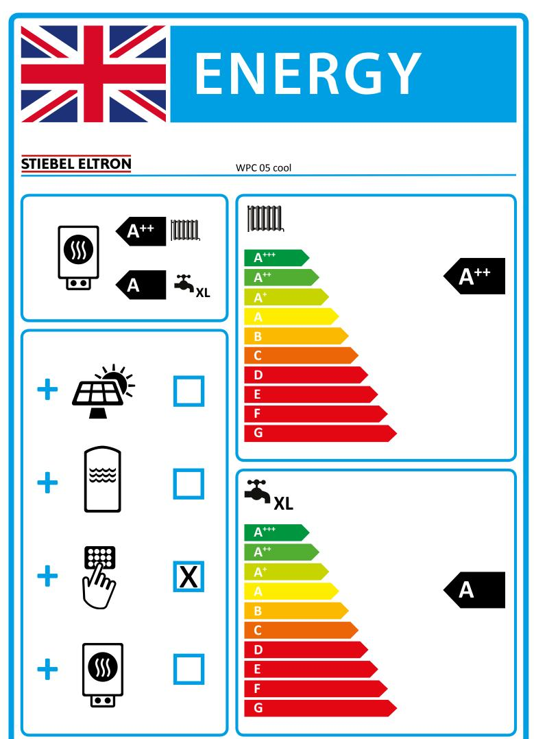
Product datasheet: Composite system consisting of room heater and temperature controller to regulation (EU) no. 811/2013 / (S.I. 2019 No. 539 / Schedule 2)
